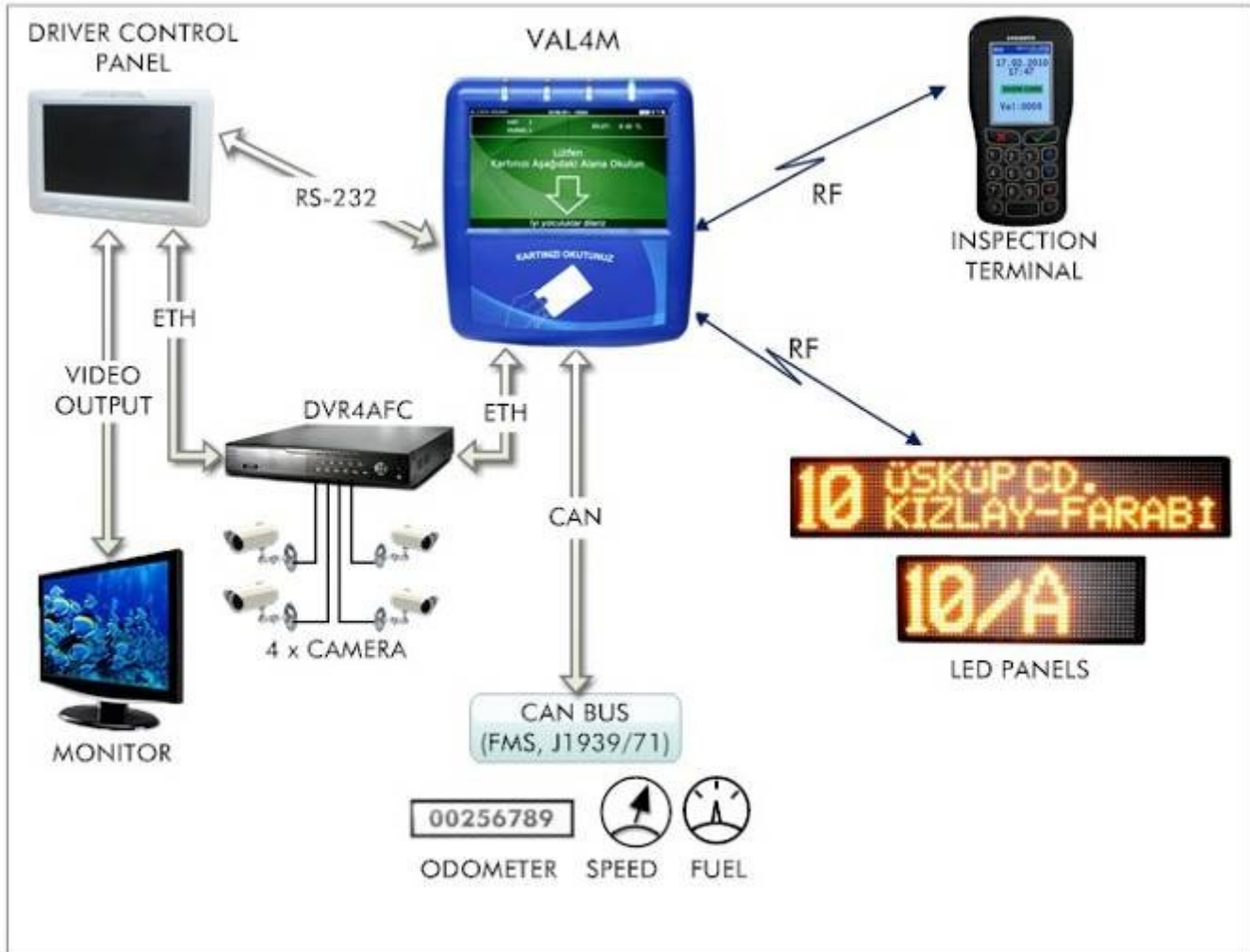
Fig 2: In vehicle AFC equipment diagram
